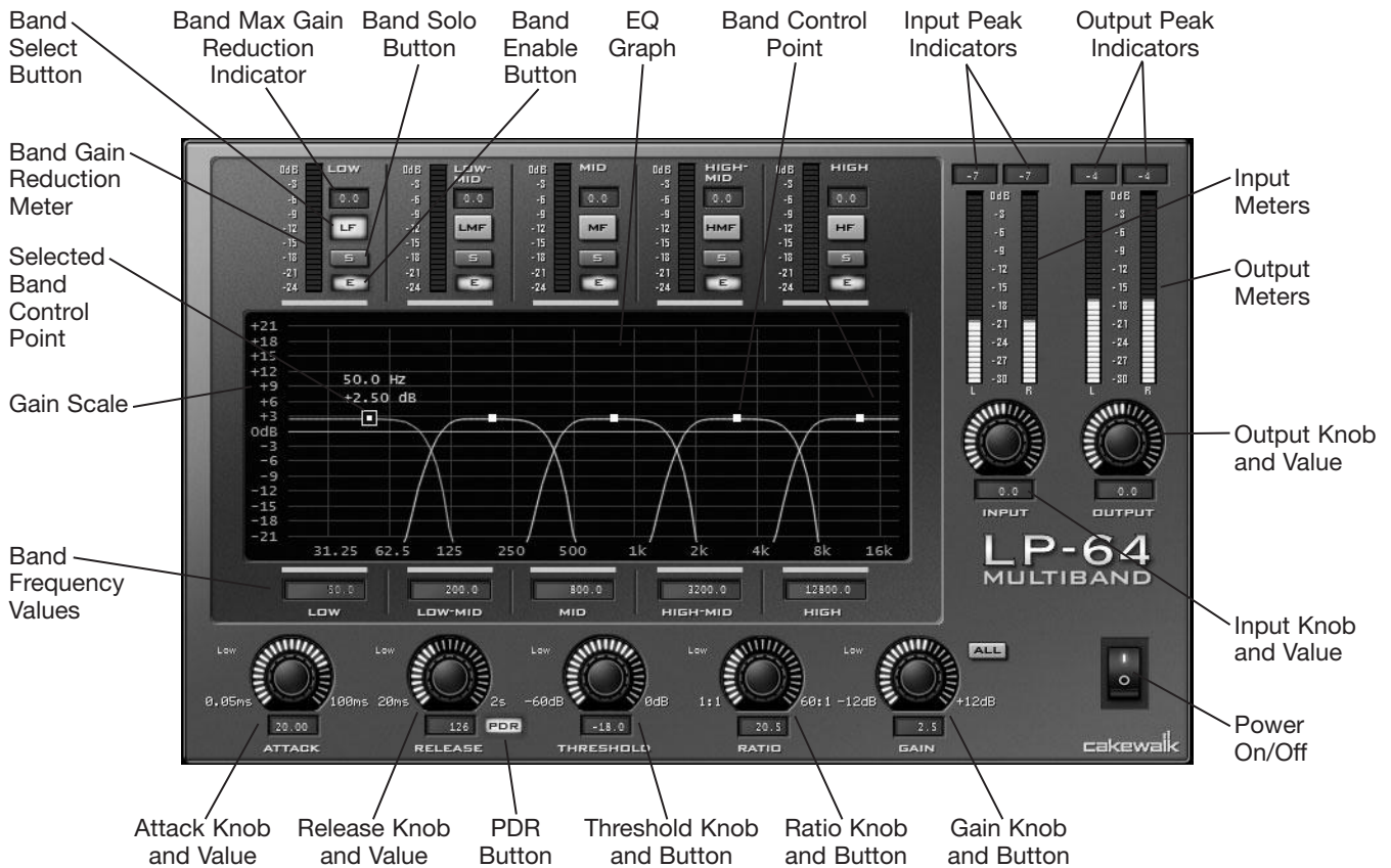
Figure 11.4 Create your own compression filters by manipulating the band parameters of the Linear Compressor.
