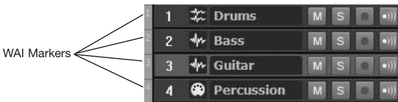
Figure 12.7 WAI markers show you which tracks and buses are being controlled by your surface.
