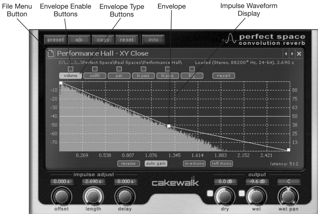
Figure 11.3 Use the Perfect Space effect to apply complex environment simulation effects to your audio data.
