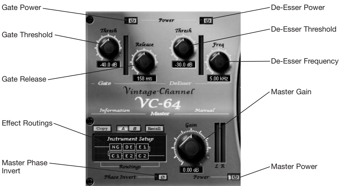
Figure 11.14 Utilize the Master, De-Esser, and Gate controls to begin working with the Vintage Channel.
