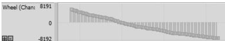
Figure 6.16 The pitch wheel is the one exception to the way controllers are displayed in the Controllers pane.
