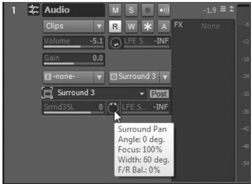
Figure 14.11 The Small Surround Panner is displayed on an aux send that is routed to a surround bus.
