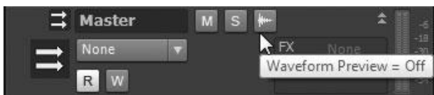
Figure 10.6 Use the Waveform Preview feature to view a real-time waveform display for buses.
