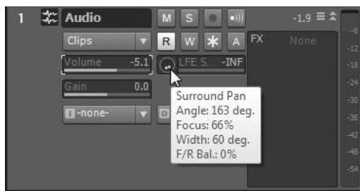
Figure 14.10 The normal Pan parameter of an audio track transforms into the Micro Surround Panner.
