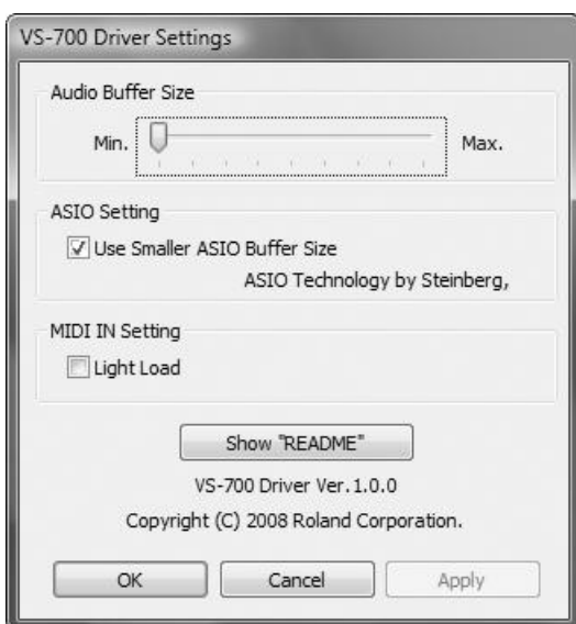
Figure 2.11 Use the ASIO control panel to adjust latency when you are using ASIO drivers.
